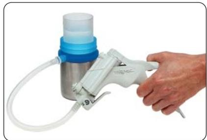
**12** When all of the sample has been filtered, detach the vacuum pump and remove the filter funnel from the rubber base. The membrane filter is now ready to be removed and placed in the petri dish containing the absorbent pad and growth media.
