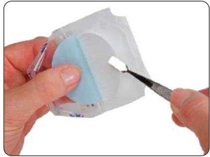
4 Peel back the transparent outer wrapper and use the sterile forceps to separate the white, gridded membrane filter from its blue backing paper and remove from the outer wrapper. Only ever grip the membrane filters at their edge.
