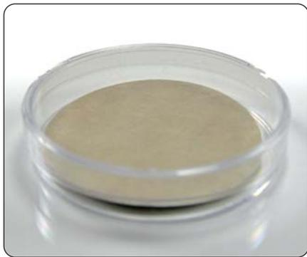
**NutriDisks** are the option most commonly used with the Wagtech Test kits. **NutriDisks** are larger than the standard aluminium petri dishes supplied in the kit but are still designed to fit into the standard petri dish rack. This allows up to 7 **NutriDisks** to be incubated at the same time.
