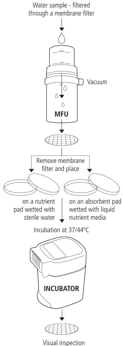
A vacuum hand pump attached to the MFU creates suction that pulls the sample water through a sterile membrane filter that sits in place in the MFU.
