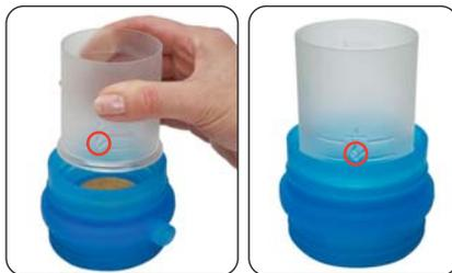
Once the flame has virtually extinguished, invert the filter funnel and silicone rubber base components of the MFU and insert into sampling cup as shown below.
