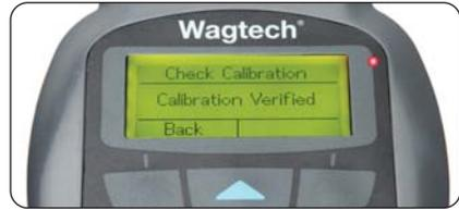
The Check Calibration function provides a simple electronic check that both thermistors are reading the same temperature as each other within a specified tolerance. If the comparison is out of range the display will show **Error 107: Validation**.
