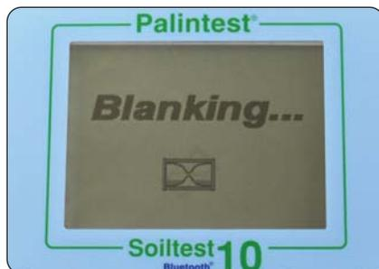
The Soiltest 10 Bluetooth will determine the absorbance due to the sample colour at all wavelengths simultaneously and store in temporary memory for use in analysis.
