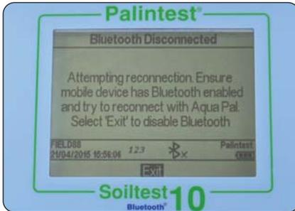
Check the Bluetooth has not been inadvertently deactivated in the mobile device settings.
