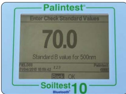
Use the up/down keys to adjust the values to match the certificate, following the order defined on the display. Press OK when the correct value is shown and the prompt will forward to the next value.
