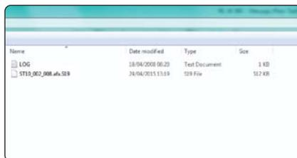
Operating software or calibration library can be updated by dragging a new version to the instrument - contact support@palintest.com for new software if this option is required. Any updates to operating software will be notified via the [www.palintest.com/know](http://www.palintest.com/know) portal.
