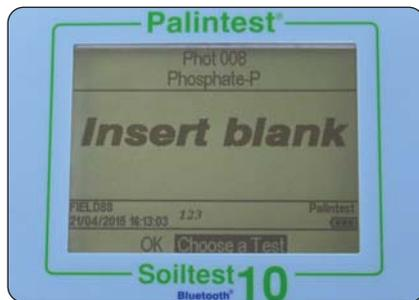
Insert the Blank cuvette and press OK.
