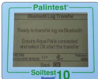
Transferring selected data will require specification of the result log window e.g. from result 40 to result 100 to be transferred selectively.
