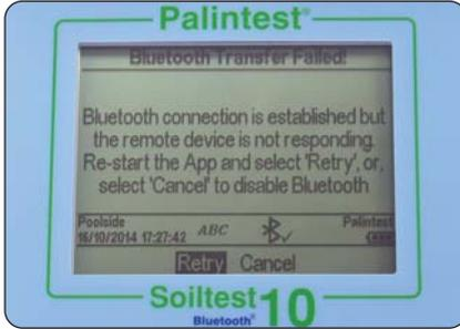
The Soiltest 10 Bluetooth is not receiving a response from the Palintest Aqua Pal app but the remote device is connected. This will appear 10s after a result transmission has started and no valid response has been received.
