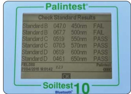
If the Check Standard Mode reports a failure, see Appendix 2 Troubleshooting for guidance or contact your local Palintest supplier.
