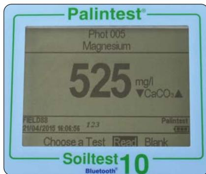
Where alternative units of expression for results are available the  $\blacktriangle$  $\blacktriangledown$  symbols will be displayed next to the current result units. Use the up/down arrows to change the units of expression as required. Values are modified automatically.
