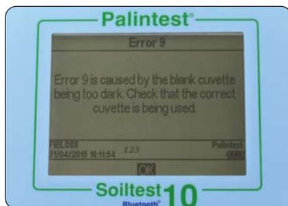
Ensure the blank cuvette is being used, not the sample plus reagent cuvette. Sample colour can be reduced by dilution with clean water; the dilution selected should take account of the expected concentration of parameter under test.
