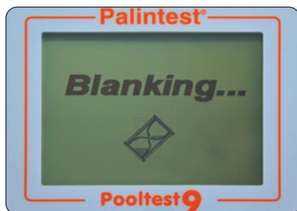
The Pooltest 9 will determine the absorbance due to the sample colour at all wavelengths simultaneously and store in temporary memory for use in analysis.
