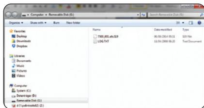
Operating software or calibration library can be updated by dragging a new version to the instrument.
