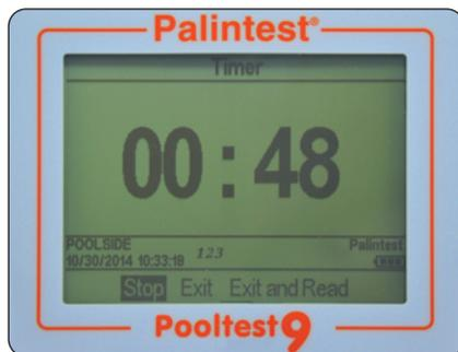
The programmed reaction time will be displayed. Press **OK** to **Start** the countdown.
