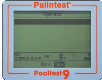
To create a new Sample ID, select Sample ID and use the up/down keys to select a blank field. Select New and press OK.
