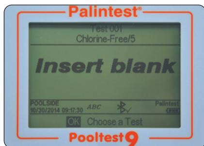
Insert the Blank cuvette and press OK.
