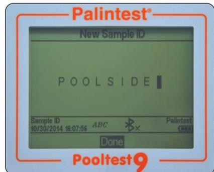
When the Sample ID is correct press the OK key to create the ID and return to the Sample ID list. The new Sample ID will be displayed in the Sample list. Choose the Sample ID to be used by scrolling through the list and pressing the OK key on the desired choice. The instrument will return to the System menu.
