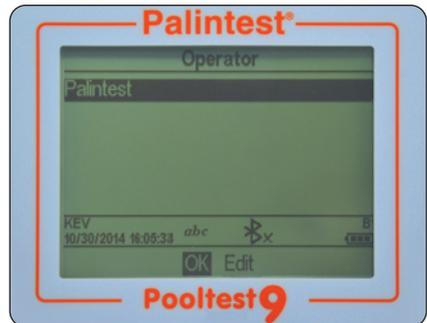
To create a new Operator ID, select Operator ID and use the up/down keys to select a blank field. Select New and press OK.
