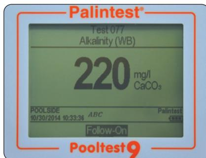
To access the Follow-on test, highlight Follow-on and press OK. The next method is automatically loaded and operated in the usual manner.
