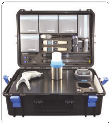
**1** Loosen the filter funnel and remove from the rubber base support. Invert the filter funnel and place it down on the clean work-surface. Also place the blue rubber base support down on the work-surface. Ensure that these items are only ever placed onto the clean work-surface.
