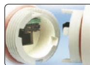
To install the new sensor, line up the tabs and 8 pins of the sensor to the instrument body. Twist ribbed collar back on to keep waterproof rating and secure sensor. The O-rings should create a watertight seal and provide some resistance when twisting.
