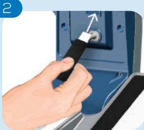
Open the arm, and insert the first of three check standards from the KEMC10 pack.
