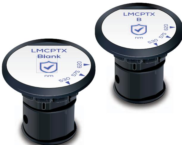
Using check standards is a simple way to verify the performance of the instrument and check that it is within calibration. Check Standards are comprised of neutral density filters in special holders. These absorb a similar level of light at all frequencies. Therefore, a single NDF can perform the same checks as the different liquid colour standards used with earlier Palintest photometers.
