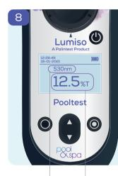
The measurement of %T (Percentage Transmission) is shown on screen.
