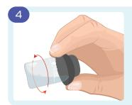
During sample testing or blanking, remove any attached bubbles by capping the tube and rotating as shown.
