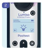
Use the up and down keys to adjust the brightness of the screen as required.
