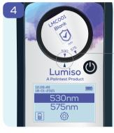
Ensure that the wavelength being checked is aligned with the mark on the Lumiso instrument
