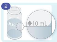
When filling tubes to the 10 mL line ensure the level is as shown
