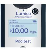
If a result is above the range of the test a '>' symbol will appear in front of the result. In this case it will be necessary to dilute the sample with deionised water and repeat the test.
