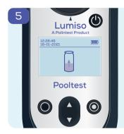
The screen will show that the blank is being measured.
