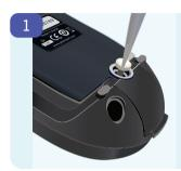
To change the batteries, first disconnect the USB lead
