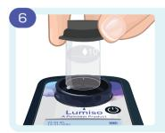
Ensure that your Lumiso Instrument is clean and dry. Place tubes in the instrument with white diamond aligned to the mark on the instrument.
