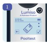
Sample readings can be tagged to indicate a sample name, project or sampling location.
