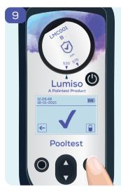
Continue, by inserting Standard B, pressing read, and comparing the result with certificate.
