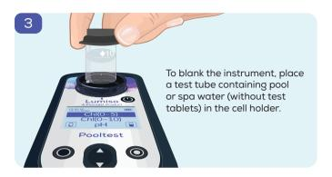
Blanking enables the instrument to set the correct zero value. This ensures the final result will be accurate, even when testing water that is cloudy or coloured.
