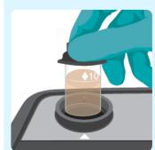
Place in cell holder and press Measure to obtain value for Colour on Pt/Co Scale.
