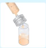
Filter 10 mL of sample through a GF/B filter .
