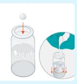
Prepare sample by adding a Coppercol No1 tablet and crush and stir.
