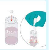
To the same sample, add a Coppercol No2 tablet and crush and stir.
