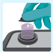
Place back in cell holder and press Measure. Total Copper concentration will be displayed. Press Finish, to scroll through Free, Total and Chelated Copper.
