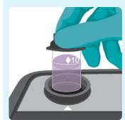
Place the prepared sample in the cell holder and press Measure to obtain the concentration of Free Copper. Then press Continue.
