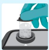
Place the tube in the cell holder and press Measure to obtain concentration of Cyanuric Acid.
