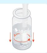
Crush any remaining particles and stir.
