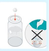
Prepare sample by adding a Cyanuric Acid tablet, but, do not crush.
