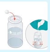
Prepare sample by adding a Hardicol No1 tablet and crush and stir.
