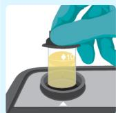
Place in cell holder and press Measure to obtain concentration of Hydrogen Peroxide.
