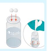
Prepare sample by adding an Acidifying PT tablet and a Hydrogen Peroxide HR tablet. Crush both tablets and stir.
