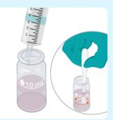
Fill to the 10 mL line with further sample and stir.
