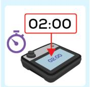
Allow timer to count down 2 minutes. The concentration of Hydrogen Peroxide will then be displayed.
