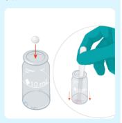
Add a Hydrogen Peroxide LR tablet to those drops. Then, crush to form a paste.
