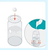
Then, prepare sample by adding an Iron HR tablet and crush and stir.
