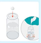
Then, prepare sample by adding an Iron LR tablet and crush and stir.
