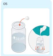
Then, add an Iron MR No2 tablet and crush and stir.
