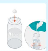
Add a Citrate IR tablet. Crush and stir until fully dissolved.
