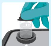
Use this to "blank" the instrument. Place in cell holder and press Blank.
