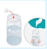
Prepare sample by adding an Iron MR No1 tablet and crush and stir.
