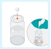
Add a Citrate IR tablet. Crush and stir until fully dissolved.
