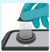
Use this to "blank" the instrument. Place in cell holder and press Blank.
