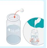
Then, add an Iron MR No2 tablet and crush and stir.
