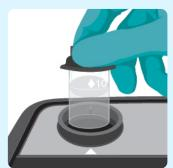
Use this to "blank" the instrument. Place in cell holder and press Blank.
