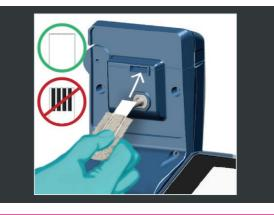
If the sensor is not fully inserted, push it in all the way using the edges of the sensor only. Do not touch the dosed chemicals on the electrode surface.
