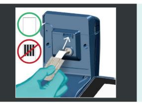
If the sensor is not fully inserted, push it in all the way using the edges of the sensor only. Do not touch the dosed chemicals on the electrode surface.
