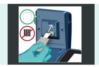
If the sensor is not fully inserted, push it in all the way using the edges of the sensor only. Do not touch the dosed chemicals on the electrode surface.
