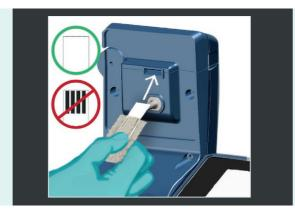
If the sensor is not fully inserted, push it in all the way using the edges of the sensor only. Do not touch the dosed chemicals on the electrode surface.
