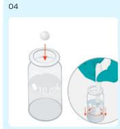
Prepare sample by adding a Magnecol tablet and crush and stir.
