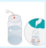
Prepare sample by adding a Nickeltest No 1 tablet and crush and stir.
