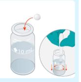
Then, add a Nickeltest No2 Tablet and crush and stir.
