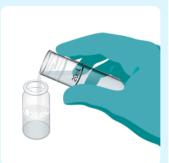
Carefully decant 10 mL of clear liquid in to a photometer tube.
