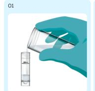
Fill a nitratest tube to the 20 mL line with sample.
