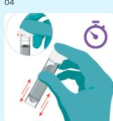
Replace screw cap and shake well for 1 minute.
