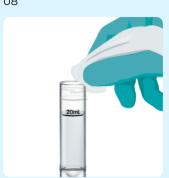
Remove cap and wipe rim to remove all traces of Nitratest powder.
