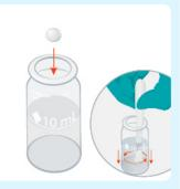
Then, add a Nitricol tablet and crush and stir.
