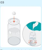
Then, add a Nitricol tablet and crush and stir.
