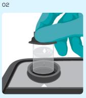
Use this to "blank" the instrument. Place in cell holder and press Blank.
