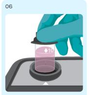
Place the tube in the cell holder and press Measure to obtain the Ozone concentration.
