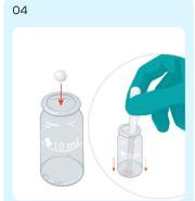
Add a DPD 4 tablet to those drops. Then, crush to form a paste.
