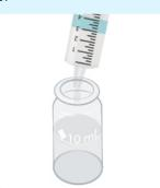
To a clean photometer tube, add a fresh 10 mL of sample.
