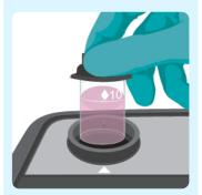
Place the tube in the cell holder and press Measure. This value will be the uncorrected concentration of Ozone. Then, press Continue.
