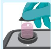
Place in the cell holder and press Measure to obtain the Ozone concentration after correction for chlorine or bromine.
