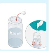
Then, add a Phosphate LR No2 Tablet and crush and stir.
