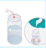
Prepare sample by adding a Phosphate LR No1 tablet and crush and stir.
