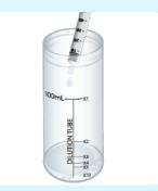
Add 0.5 mL of sample to a dilution tube. Then fill to 100 mL mark with deionised water. Replace cap and shake well to mix.
