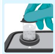
Place in cell holder and press Measure to obtain concentration of Salt (sodium chloride).
