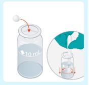
Prepare sample by adding an Acidifying CD tablet and crush and stir.
