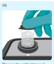
Place in the cell holder and press Measure to display the concentration of Sulfate.
