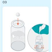
Prepare sample by adding a Sulfate Turb tablet and crush and stir.
