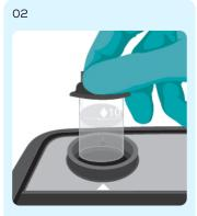
Use this to "blank" the instrument. Place in cell holder and press Blank.
