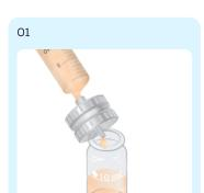
Filter 10 mL of sample through a GF/B filter .
