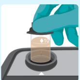
Use this to "blank" the instrument. Place in cell holder and press Blank.
