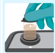
Place in cell holder and press Measure to obtain value for Turbidity. Please note: This not a nephelometric measurement.
