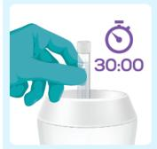
Place in water bath and leave for exactly 30 minutes at  $100^{\circ}\text{C}$ .
