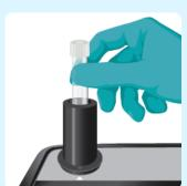
Without delay, place tube in cell holder and press Measure to obtain the concentration of Urea.
