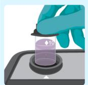
Place the tube in the cell holder and press Measure to obtain the concentration of Zinc.
