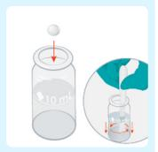
If chlorine is present, add a Zinc-Dechlor tablet and crush and stir. Otherwise, skip this step.
