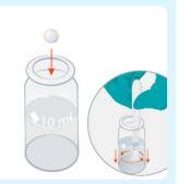
Prepare sample by adding a Phenol Red tablet and crush and stir.
