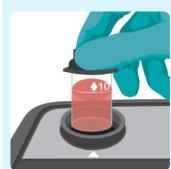
Place the tube in the cell holder and press Measure to obtain the pH value.
