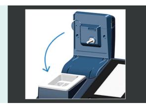
Total Bromine is measured using Palintest's BRS sensors for concentrations of bromine ranging from 0.2 mg/L - 10 mg/L across the temperature range of 5 - 30 °C.
