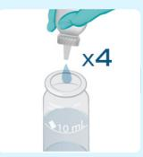
Prepare the sample by adding 4 drops of the Fluoride Liquid Reagent and stir to mix.
