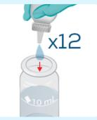
Prepare sample by adding 12 drops of Hardicol liquid buffer and stir.
