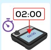
Allow timer to count down 2 minutes. The result for Total Hardness will be displayed.
