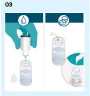
Prepare sample by adding two drop of Mn HR liquid or a Mn HR No2 tablet.
