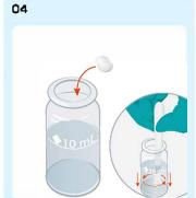
Then, add a Manganese HR No1 tablet. Crush and stir until fully dissolved.
