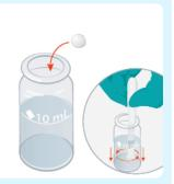
Then, add a Manganese No2 tablet and crush and stir.
