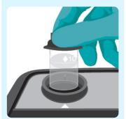
Use this to "blank" the instrument. Place in the cell holder and press Blank.
