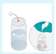
Add one Manganese LR No 1 tablet and crush and stir.
