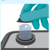
Add the tube to the photometer and press measure. The result is displayed as mg/L Mn.
