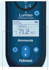
The measurement of %T (Percentage Transmission) is shown on screen.
