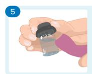
Ensure tubes are dry on the outside before placing them in the instrument
