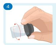
During sample testing or blanking, remove any attached bubbles by capping the tube and rotating as shown.
