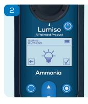
Use the up and down keys to adjust the brightness of the screen as required.
