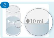
When filling tubes to the 10 mL line ensure the level is as shown
