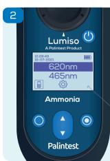
The wavelengths of light the instrument uses are shown in nanometres (nm).
