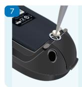
Secure the captive screw so that it gently holds the cover in place, do not overtighten the hold.
