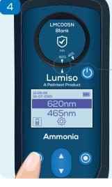
Ensure that the wavelength being checked is aligned with the mark on the Lumiso instrument.
