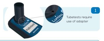
Please see section **How to Select and Perform a Test** for details of Tubetests **Blanking**.
