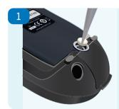
To change the batteries, first disconnect the USB lead
