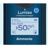
If a result is above the range of the test a '>' symbol will appear in front of the result. In this case it will be necessary to dilute the sample with deionised water and repeat the test
