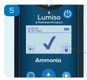
The instrument will measure the blank and show when this has been successful.
